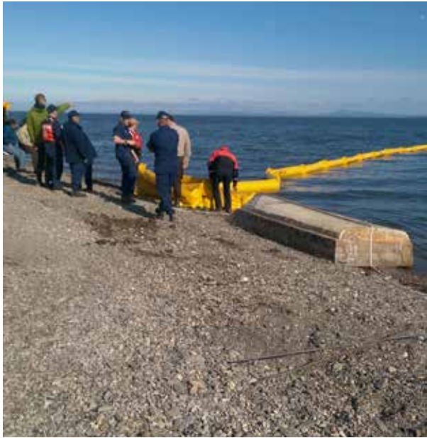
Figure 7. Deployment of boom during a Geographic Response Strategies testing exercise, June 2015 in Kotzebue, Alaska.
