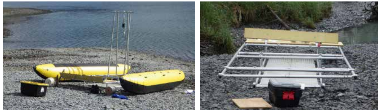
Figure 2. The cataraft coring platform is built on the beach of a small lagoon within Kenai Fjords National Park. Coring platform and NPS skiffs are set to cast off and head to the first coring target (top). Aluminum frame and 18-foot pontoons are assembled and inflated in preparation for launch (bottom left and right).
