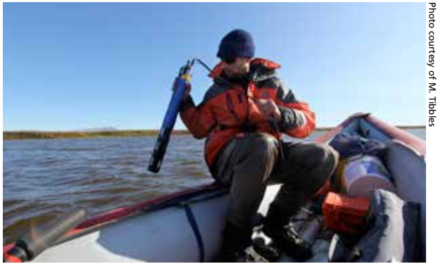
Figure 3. Measuring water chemistry (e.g., salinity, temperature, dissolved oxygen) at Aukulak Lagoon, Cape Krusenstern National Monument.
