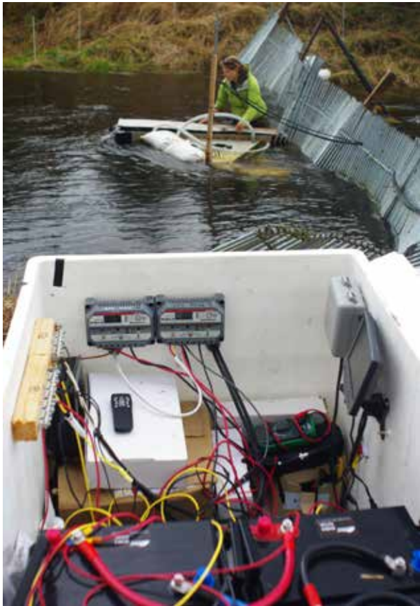
Figure 7. National Park Service biologist Lisa Schomaker performs regular maintenance on the video weir on Silver Salmon Creek. The fence on the right forces salmon through a chute in front of an underwater camera. The camera is powered by solar panels and controlled by the electronics in the foreground.
