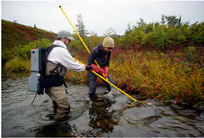
Figure 10. J. Johnson (ADFG) and Sarah O'Neal (FRC) fish with a backpack electrofisher, which sends a slight electrical charge through the water to attract and momentarily stun fish so they can be easily netted.
