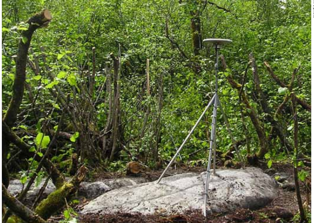
Figure 5. This Geographic Positioning System (GPS) site in Glacier Bay is designed to precisely and continuously measure bedrock movement caused by isostatic uplift. Visual impact was reduced by concealing minimal equipment within a patch of vegetation.
